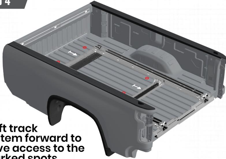
Shift track system forward to have access to the marked spots.
