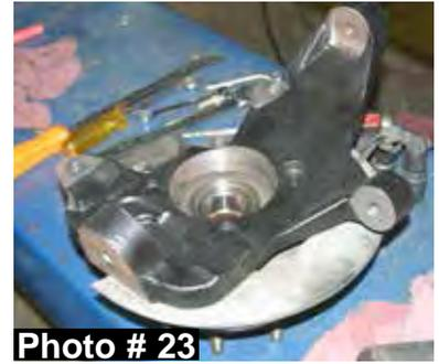
34. Install the new Skyjacker steering knuckles & attach the upper & lower control arms to the steering knuckle using the OEM hardware. The outer tie rod end will install from the top instead of from the OEM bottom position. (See Photo # 24)
