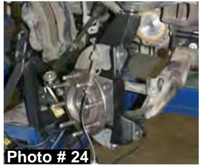
35. Reinstall the brake rotor & brake caliper. Attach brake line to the side of the steering knuckle using the 5mm screws provided. **Note:** Some models have a OEM 6mm bolt that can be reused. Attach the ABS line to the upper control arm using the OEM bolt with the plastic clips provided. (See Photo # 25)
