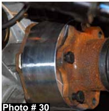
Driver side shown with 3.35" cv-shaft spacer.
